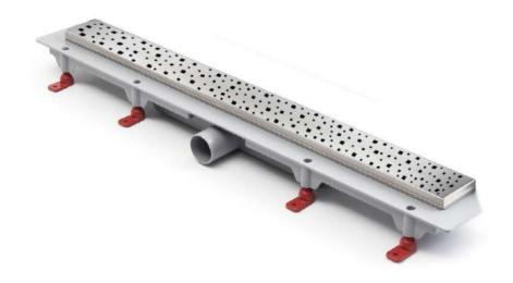
The package includes installation instructions, self-adhesive waterproofing membrane, adjustable legs, nylon plugs and screws.
