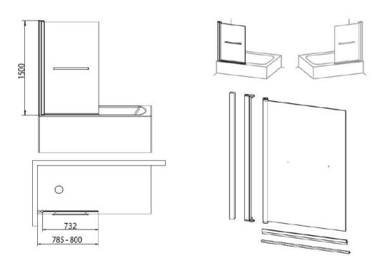
Adjustment range for compensating for 1 wall: 15 mm (-0mm / +15mm)
